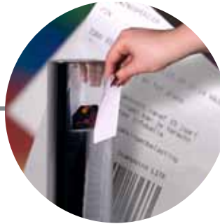
Barcode scanner triggering to open the gate
